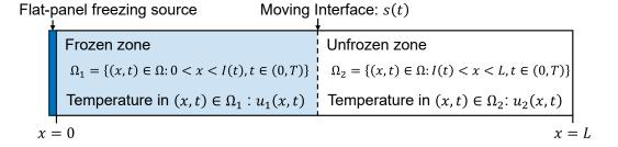
Fig. 1 Schematic of 1D heat conduction with two phases
